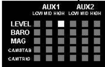
Depending on your configuration, you can easily activate/deactivate options via 2 switches on your RC TX. The 2 switches correspond to (AUX1), typically RX ch5 and, RX channel 6 (AUX2). In Version 2.0 and later, two additional channels (AUX3 & 4) may also be used if you are using PPM composite receiver (see Other Neat Stuff section below)
